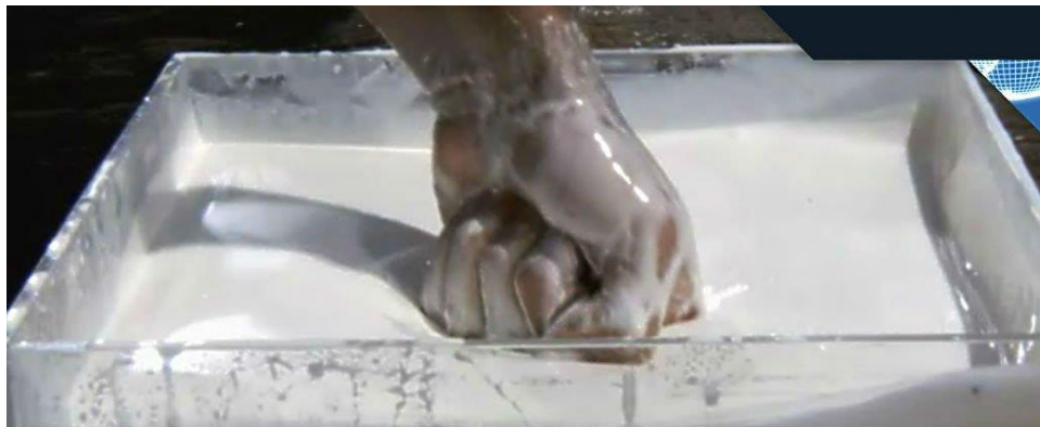
Figure 6: Non-Newtonian Fluid Taking Impact from Punch
